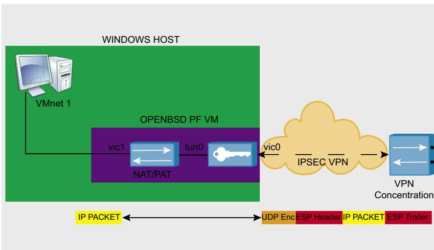
Figure 11. VPN encapsulation on the Virtual Router
