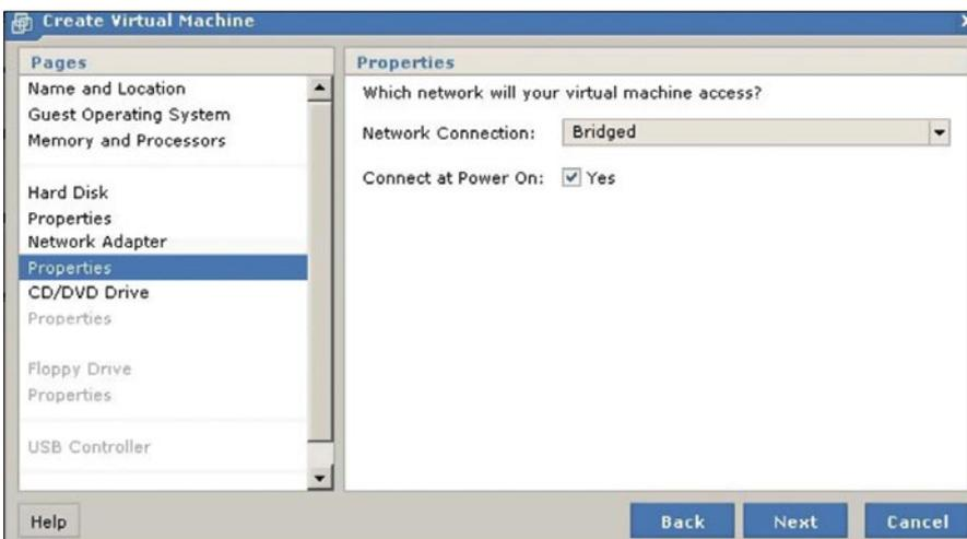
Figure 8. VMware Server: Virtual Machine network connection
