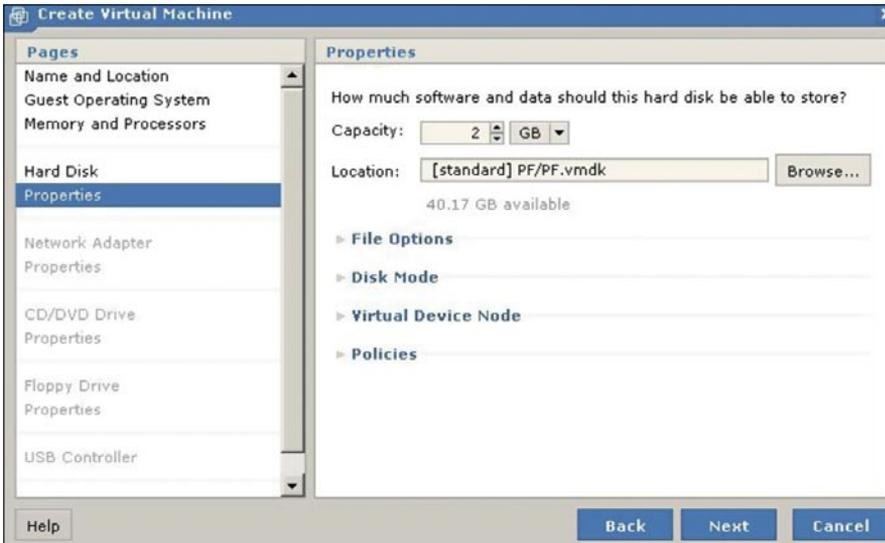
Figure 7. VMware Server: Virtual Machine disk configuration
