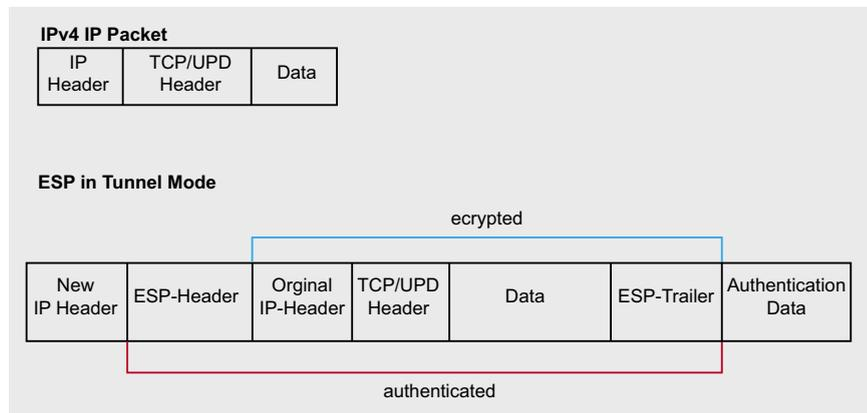
Figure 2. IPv4 datagram before and after ESP encapsulation in tunnel mode
