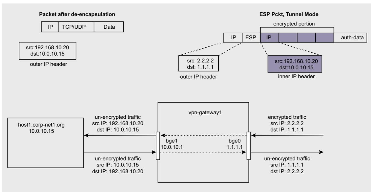
Figure 3. Traffic flow for an ESP packet
